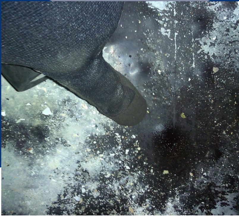
Corrosion Barrier "Blister": HCL permeation to Ash in E-Glass = CO2
