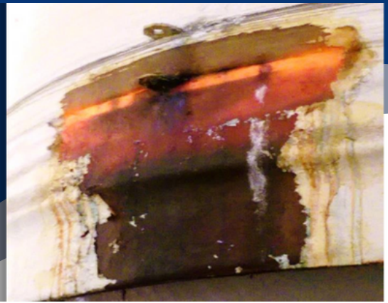
Exterior impact (Above) causes Inner fracture (Below)
